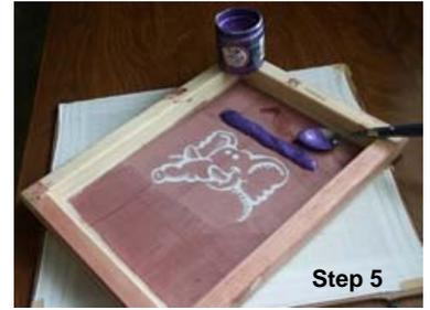
Once all fabric is printed, remove excess ink from the screen with a scrap piece of card or spoon. Wash the remaining residue with warm water. To remove the screen filler stencil, apply Comet cleanser to both sides of the wet screen, scrub lightly with a soft bristle brush and allow to stand for several minutes. Scrub a bit more and rinse with a stream of hot water; repeat if necessary to remove heavier areas. Once dry, the screen is ready for another stencil.
