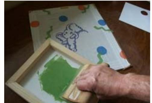
**Step 8** - After printing, remove excess ink from the screen, untape paper stencil and clean screen with warm water. Note: Some residual staining of screen mesh is normal.
