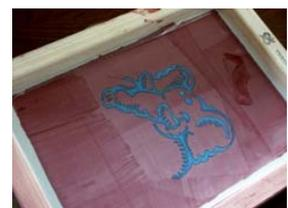
Allow the screen filler to dry completely. Once the filler is dry, rinse the screen in cold water. Use a sponge to softly massage stubborn areas to completely clear the screen in image area. When the screen is dried, apply screen filler with a brush to modify the design or to block out margin areas so that the screen is completely blocked in non-image area. The screen is ready to print once everything is dried.
